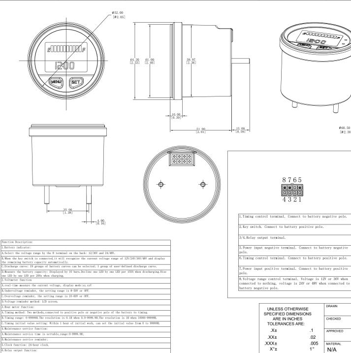
A. Battery capacity ≥10%, relay will be NC. B. Battery capacity <10% , relay will be NO.
